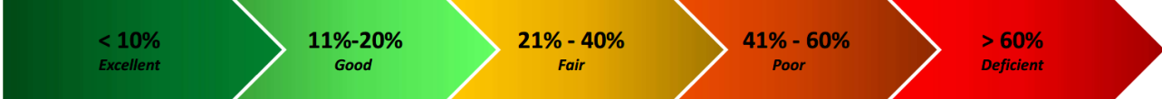
The lower an Asset’s FCI value, the better the building’s overall condition is assumed to be.
